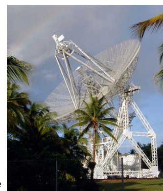
The ALTAIR (Advanced Research Project Agency (ARPA) Long Range Tracking and Identification Radar) is an Army operated radar located on the island of Kwajalein in the western Pacific. It has two missions, Anti-Ballistic Missile (ABM) testing in support of the Western Space and Missile Center (WSMC) and space surveillance. Source: Federation of American Scientists.
