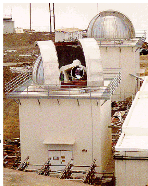
Right: The ground-based electro-optical deep space surveillance system (GEODSS) is an optical system that uses a low-light-level TV camera, computers, and large telescopes. GEODSS tracks objects in deep space, or from about 3,000 NM out to beyond geosynchronous altitudes. GEODSS requires nighttime and clear weather tracking because of the inherent limitations of an optical system. There are currently three operational GEODSS sites with coverage areas as follows: Socorro, New Mexico (165W-050W); Maui, Hawaii (140E-010W); and Diego Garcia, Indian Ocean (010E-130E). Each site has three telescopes, allowing GEODSS to track three objects simultaneously. Source: Federation of American Scientists.
