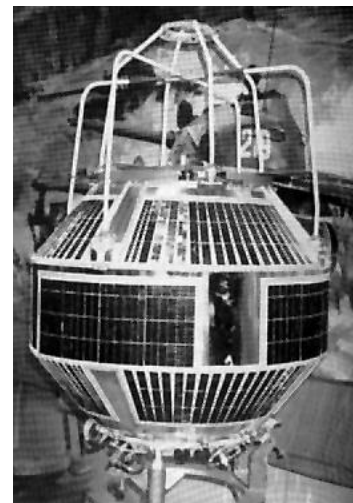
A Strela 1 store-and-forward communications satellite. Cosmos 2251 had a similar appearance. Image: www.astronautix.com .
