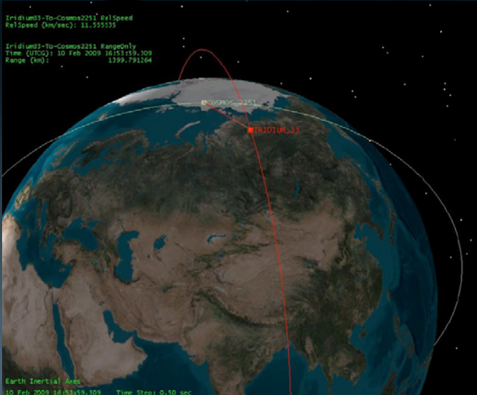
Graphic demonstrating how the orbits of Iridium 33 and Cosmos 2251 intersected at the time of collision. Courtesy: Analytical Graphics, Inc. (AGI).
