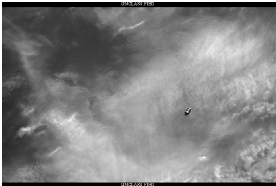
An image taken by XSS-11 of its spent Minotaur upper stage at a distance of approximately 500 meters. Photo: USAF.
